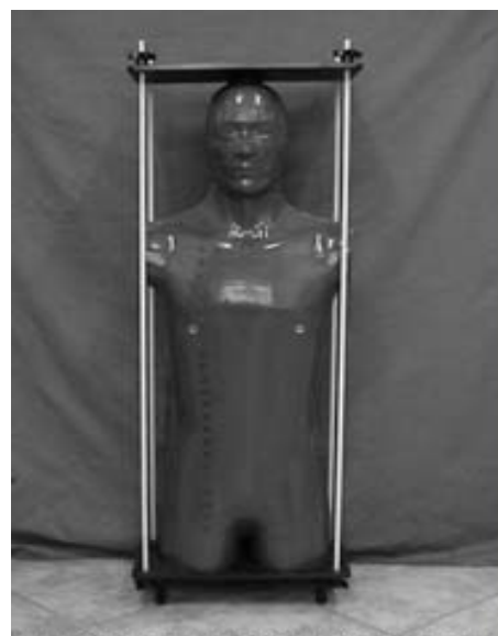
Figure 1. Alderson Rando phantom.
